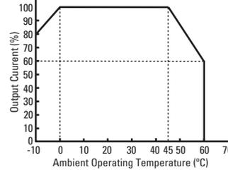
Condition Natural Air Cooling (Operating Temperature means temperature in surrounded PS5R.)
